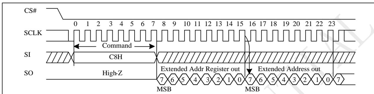
Figure 10-9a Read Extended Address Register Sequence (QPI)
