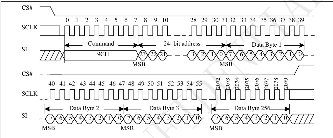
Figure 10-37a Buffer Write Sequence (QPI)
