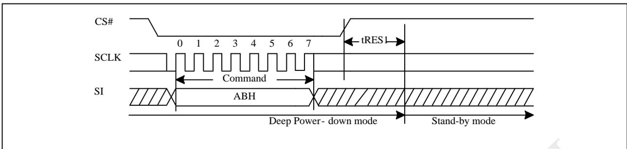
Figure 10-43c Release from Deep Power-down (RDP) Sequence (QPI)
