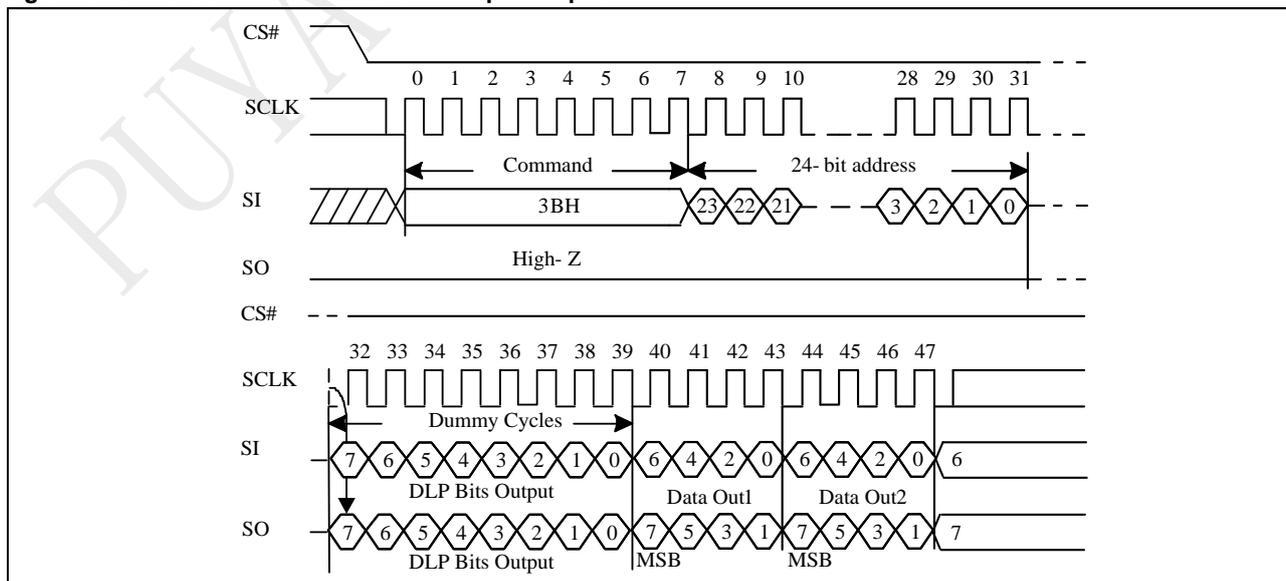
Figure 10-25b 4IO Read with DLP bits output Sequence
