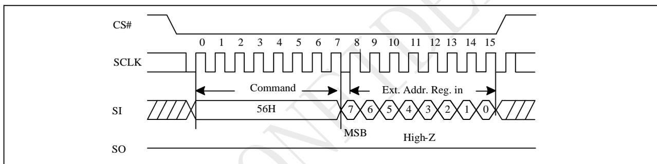
**Figure 10-10a Write Extended Address Register Sequence (QPI)**
