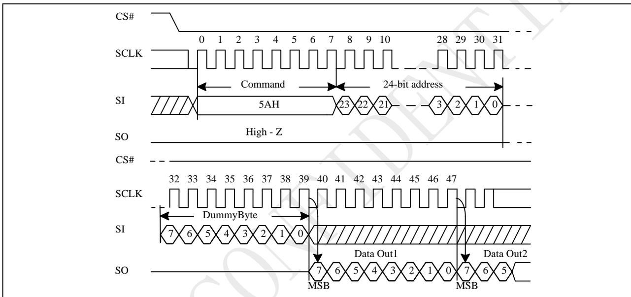
Figure 10-60a Read Serial Flash Discoverable Parameter (RDSFDP) Sequence(QPI)
