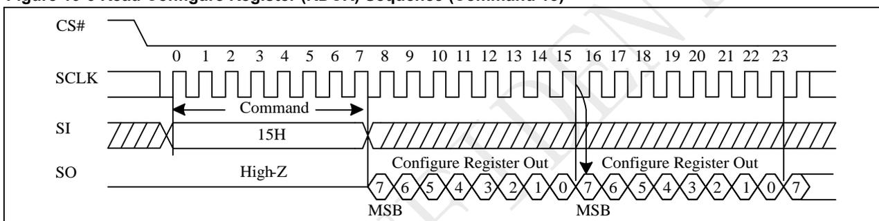
Figure 10-6a Read Configure Register (RDCR) Sequence (QPI)
