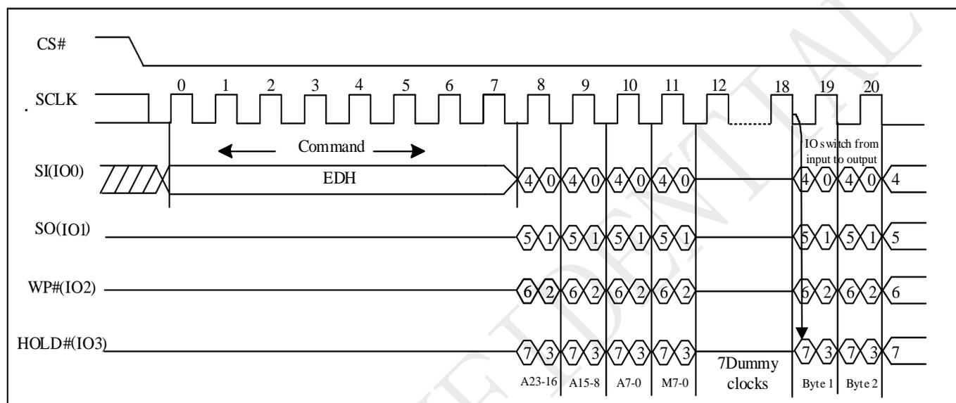
Note: 1. Hi-impedance is inhibited for the mode clock cycles. 2. M[5-4] = (1,0) is inhibited.
