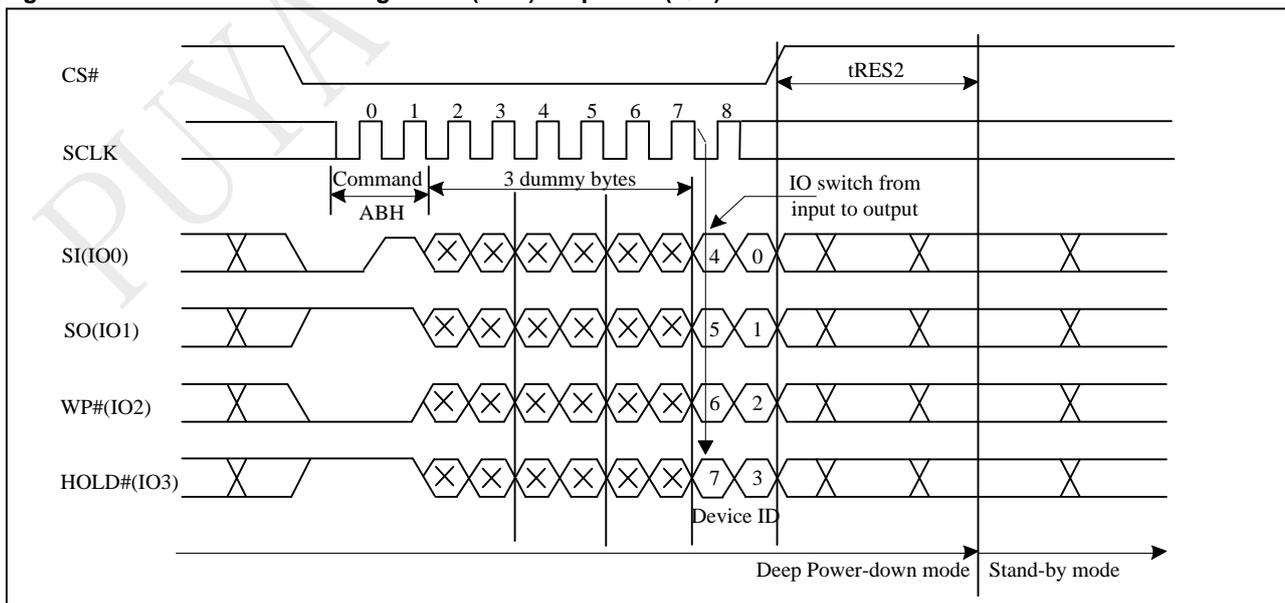
Figure 10-43b Release from Deep Power-down (RDP) Sequence (Command AB)
